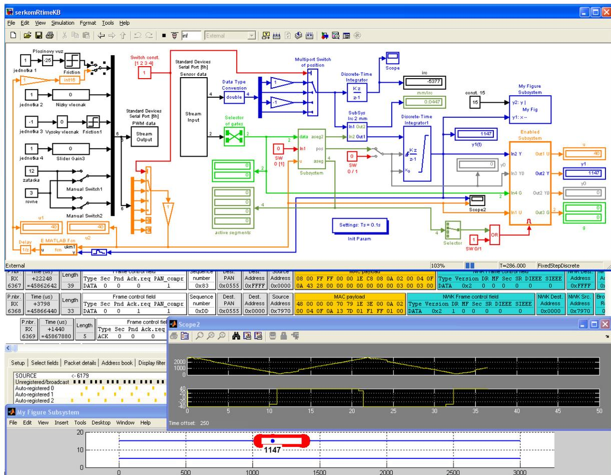
Figure 7: Screenshot of the real-time running Simulink model on control computer: Simulink model (in front and on the top); history of ZigBee frames and packets (in the background in the middle); on-line position and control action scope and simple visualization figure (at the bottom)
