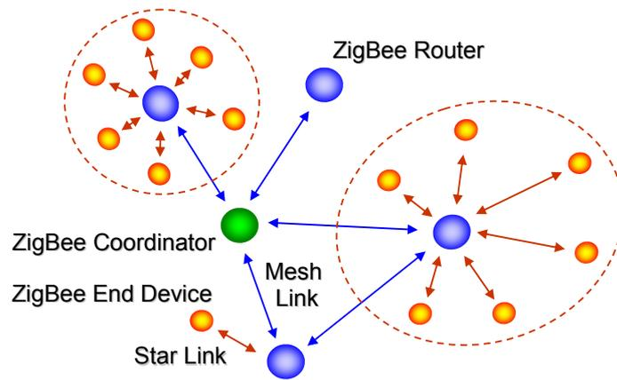
Figure 2: ZigBee network model (network topology)
