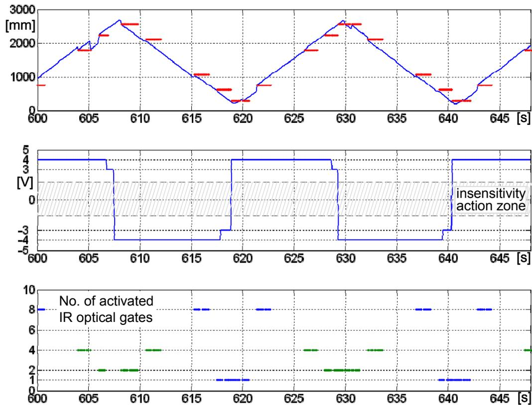
Figure 10: Control process of one movable unit: time histories of position (on the top), control actions (in the middle), activations of optical gates (at the bottom)
