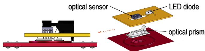
Figure 5: Optical sensor unit for position monitoring
