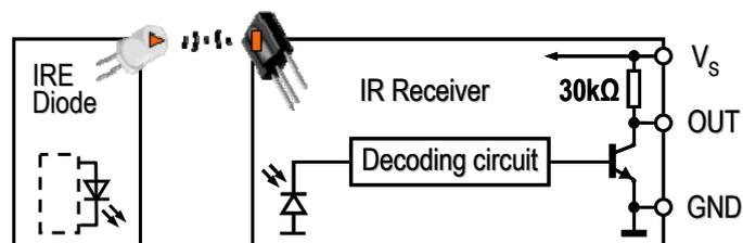
Figure 6: Circuit scheme of optical gate
