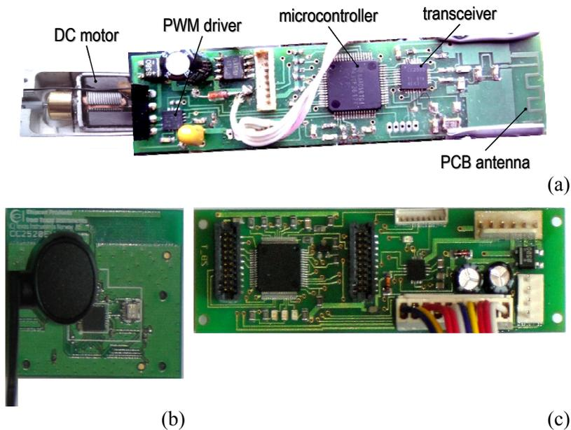
Figure 4: The boards with communication transceiver together with power-drive control of DC motor (a) – all in one solution including PCB antenna; (b) and (c) combined solution with separate boards: (b) – board of transceiver and external antenna, (c) – board of microcontroller and drive control
