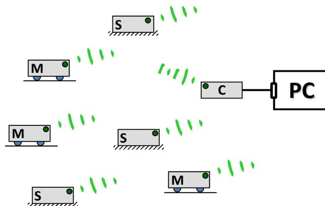
Figure 1: Distributed mechatronic system with several movable (M) and stationery (S) units and one unit for wireless communication coordination (C) connected to the control computer (PC)
