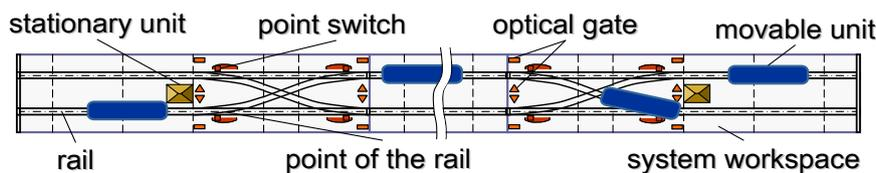
Figure 3: Mechatronic manipulation system
